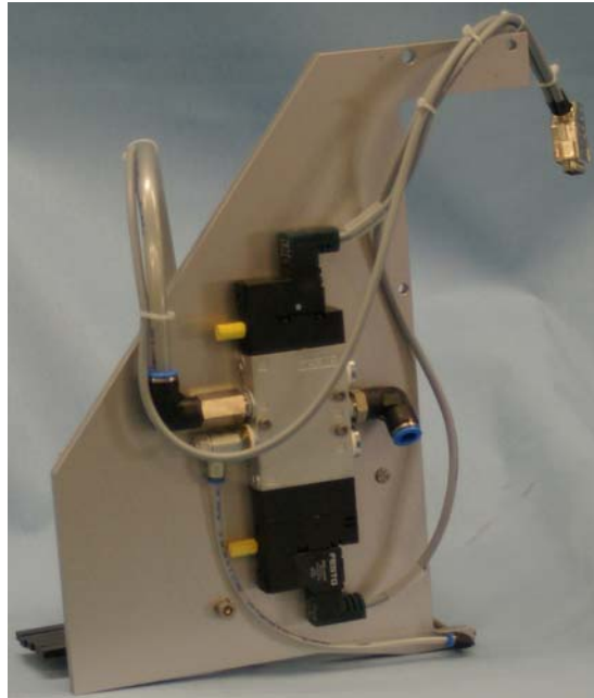
Fig. 5: The pressure valve is located on the back side of the base plate.
